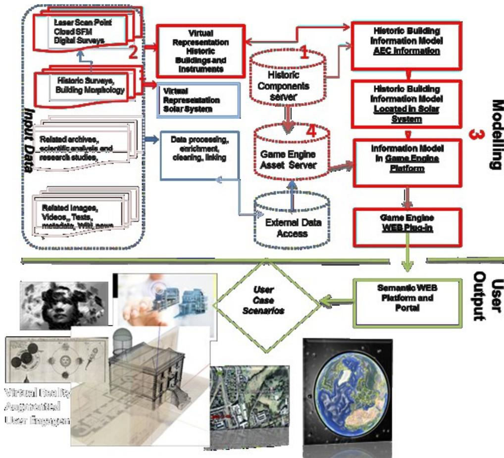
System architecture for virtual Armagh Observatory
