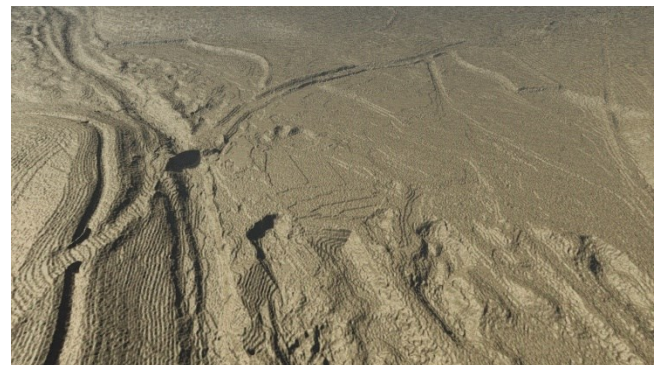
Burrator reservoir bed VR-converted sonar scan.
