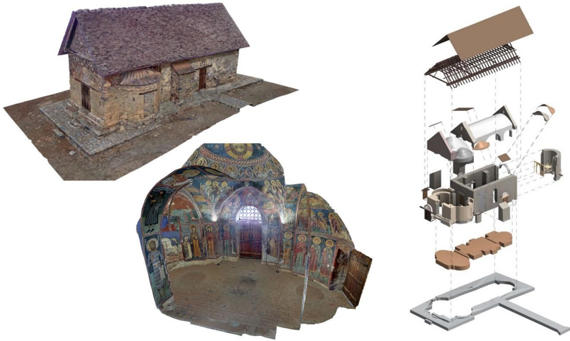
3D models and exploded HBIM model of the World Heritage site of Asinou church in Nikitari, Cyprus
